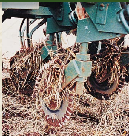
PICTURE 29: Careful selection of no-till equipment is essential. Soil type and moisture conditions have a big influence on planter performance.
