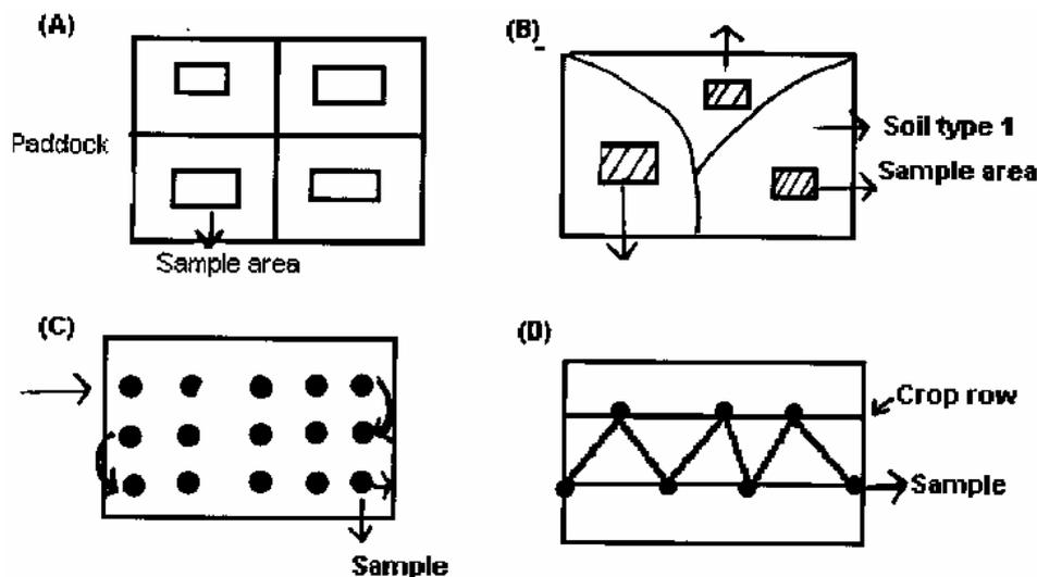
Figures A and B show paddock and sample area (Ref: Reuter and Robinson). Figures C and D show method of sampling.
