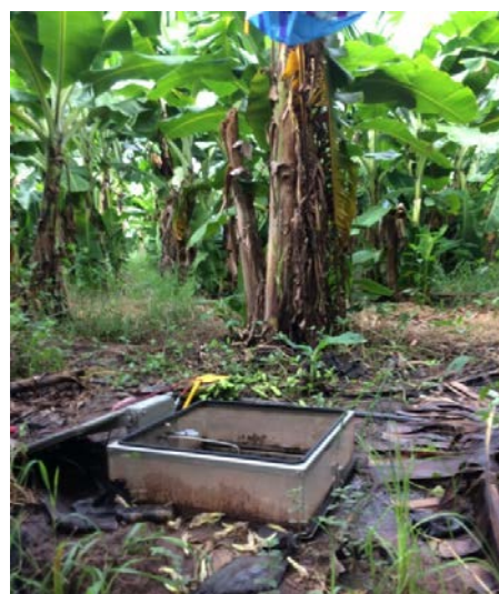
A soil gas exchange chamber in the banana gas emission trial, Kununurra, WA
