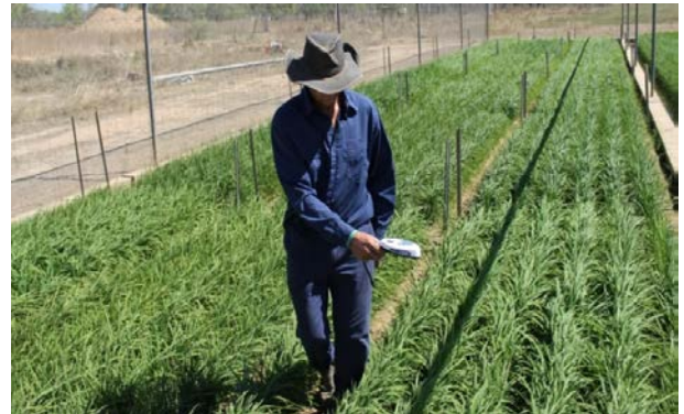
Sensing leaf colour using a portable crop sensor at 35 days after sowing
