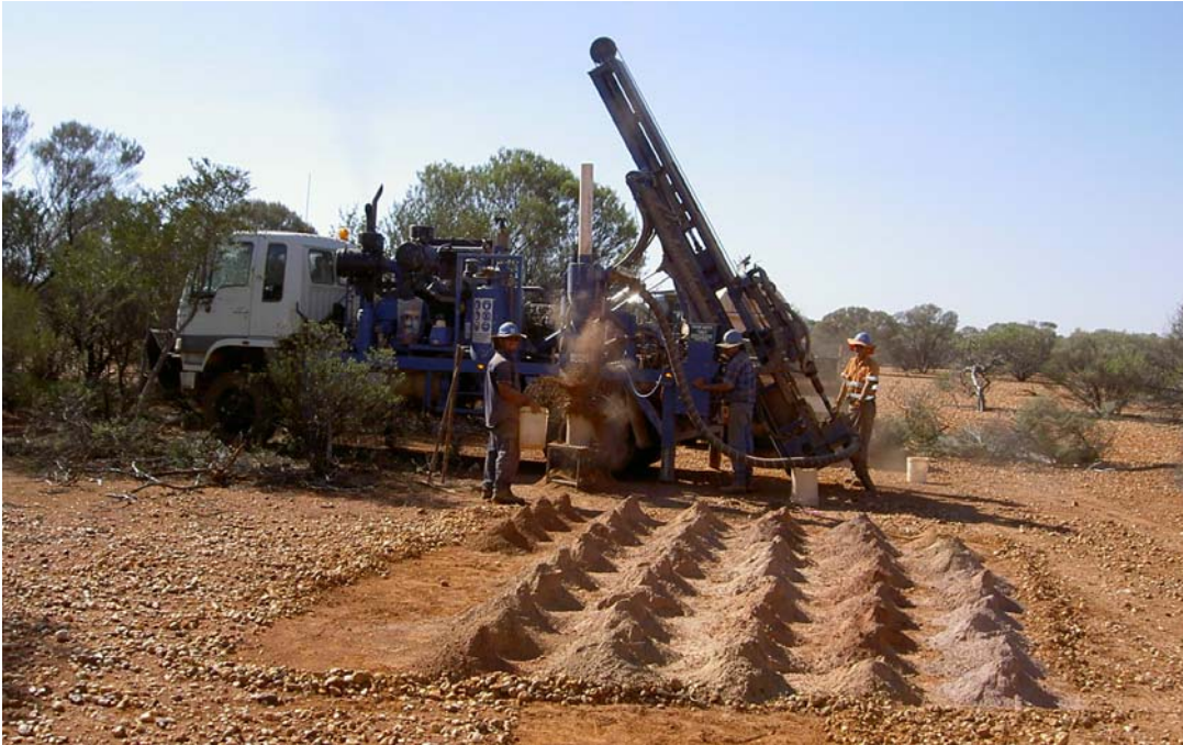
Figure 5: Aircore drilling and sampling operation.
