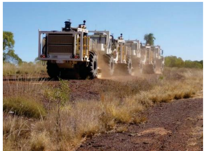
Vibroseis trucks alongside the Barkly Highway, Queensland, working on the South Nicholson Basin seismic line
