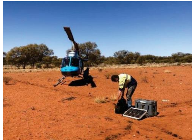
Installing Magnetotelluric data collection equipment in the NT to better understand geological structure deep below the ground.
