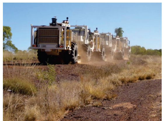
Figure 8 Vibroseis trucks alongside the Barkly Highway, Queensland, working on the South Nicholson Basin seismic line.
