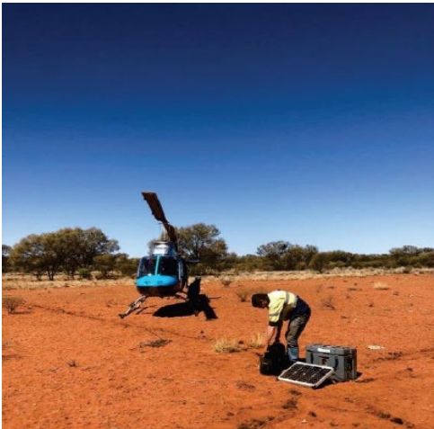
Figure 7 Installing Magnetotelluric data collection equipment in the Northern Territory to better understand geological structure deep below the ground.
