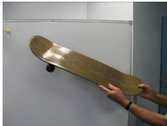
A skateboard made using hemp and flax fibres
