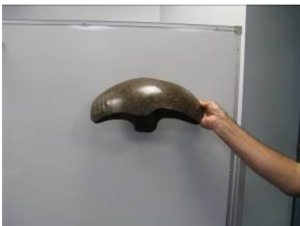
Motorbike fender made from hemp fibres and resin
