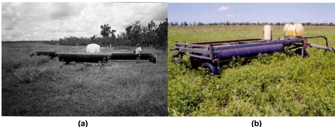
Figure 1. Carpet rollers – (a) multiple and (b) single roller designs
