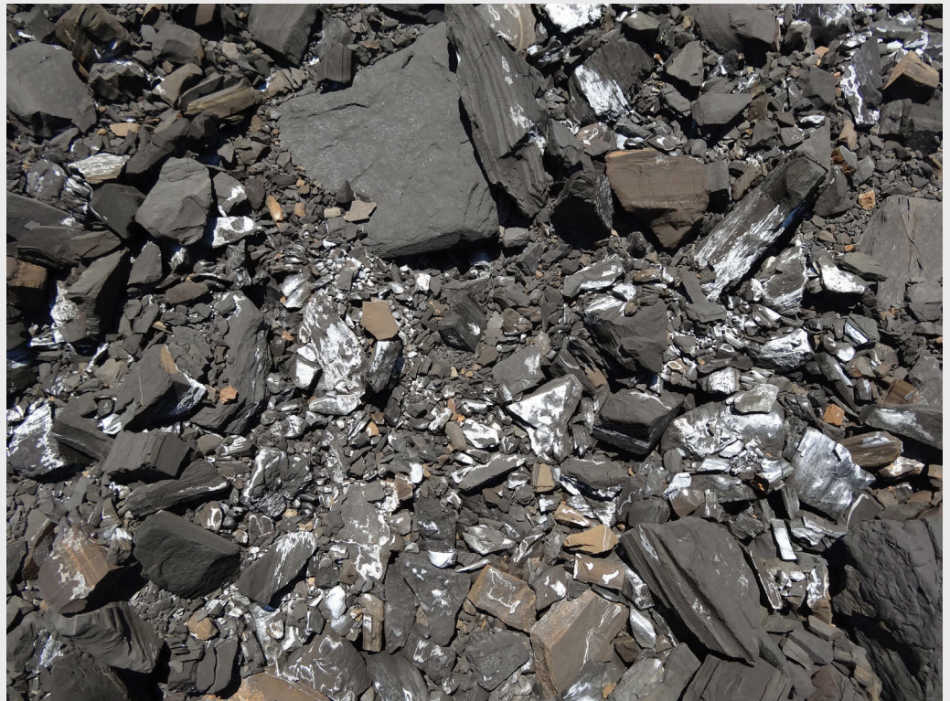
Oxidisation of potentially acid-forming rocks
