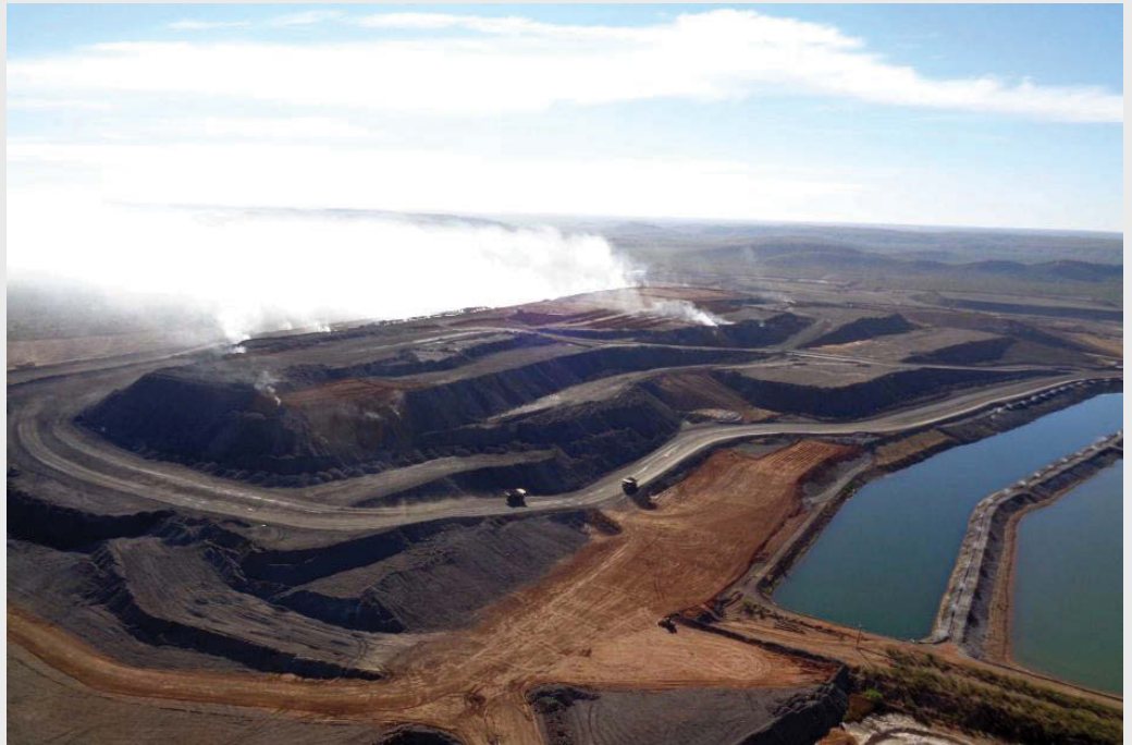
Aerial view of combustion at the Northern Overburden Emplacement Facility Source: ABC
