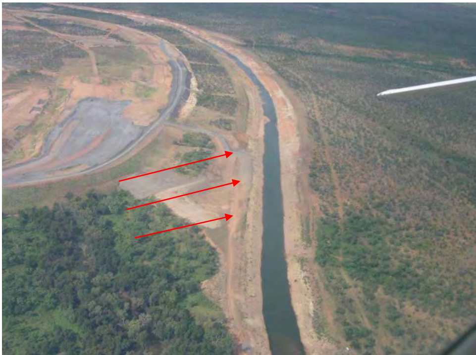
Plate 42 - The broad and denuded flowpath (marked by arrows) between the cut-off remnant river channel (left) and the diversion channel (middle of the photograph) (May 2010).
