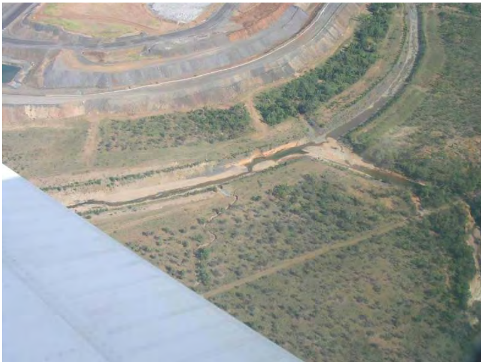
Plate 46 - The scale of erosion of the Barney Creek diversion channel's southern bank opposite the Surprise Creek entry point is clearly visible from the air (in May 2010)
