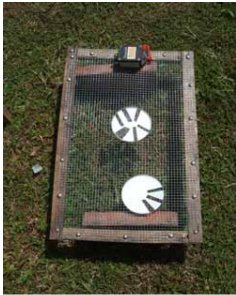
Figure 2. DS treatment: filter paper disks with urediniospores placed onto a wire grid platform and exposed to global irradiance
