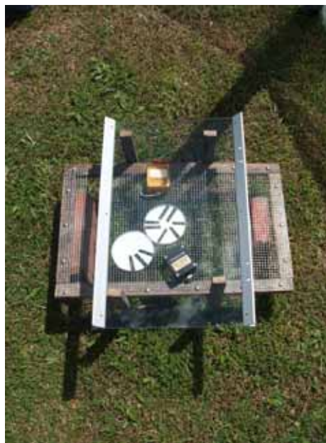
Figure 3. UV treatment: filter paper disks with urediniospores placed onto a wire grid platform and exposed to solar radiation beneath a UV filter
