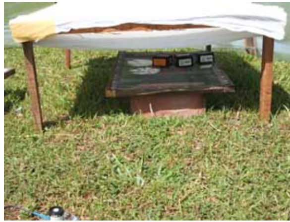
Figure 4. CH treatment: filter paper disks with urediniospores placed onto a wire grid platform and exposed to diffuse solar radiation beneath cheesecloth (shaded control)
